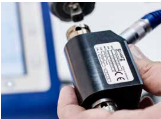
Torque and angle sensors with rotating shaft
