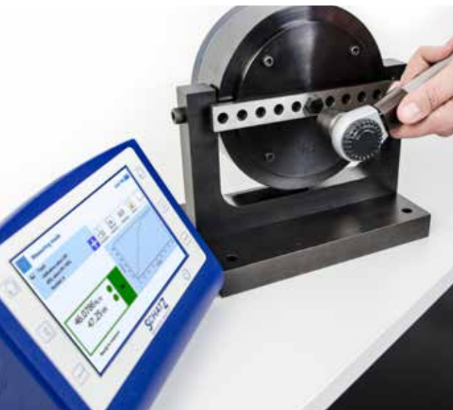
A handheld torque/angle sensor and a clamping force sensor are connected for testing.
