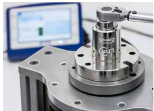
Static flange-mount sensors can be used for adaptation to torques from 10 N-m to 1000 N-m.
