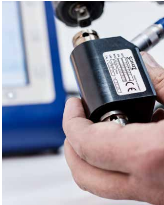
The torque/angle sensor is fitted between the male square drive of the driver and the female square drive of the socket.
