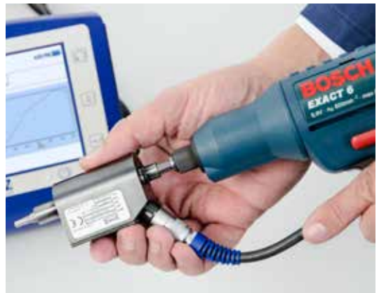
Miniature torque and angle sensors
