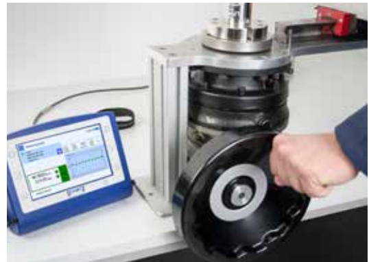
The applied torque is gradually raised with the hand crank mechanism.
