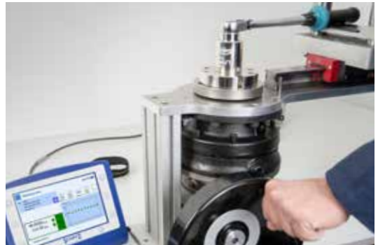
A hand crank mechanism is used to apply the torque for testing the handheld torque wrench.
