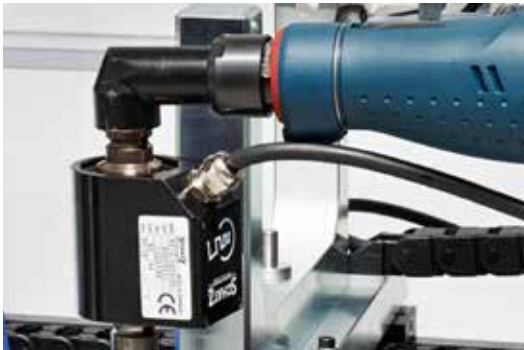
The torque/angle sensor is fitted between the male square drive and the socket.
