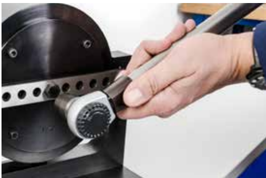
The torque, angle and clamping force need to be measured to check the bolt.
