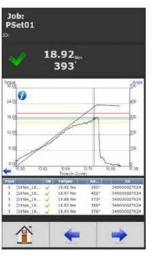
View curve results in real time or view stored results. As many as 10,000 curve results can be stored in memory.
